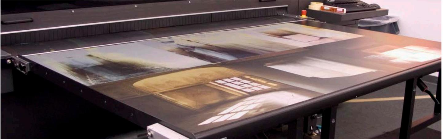
printing six 24" x 24" images on aluminum using a Vutek uv flatbed printer
